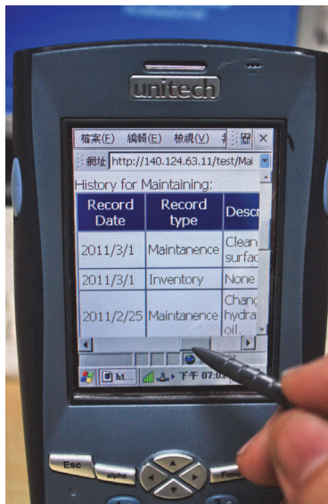
Fig. 7. Displayed maintenance staff member entered the result of inspection, edited the description in the PDA.
