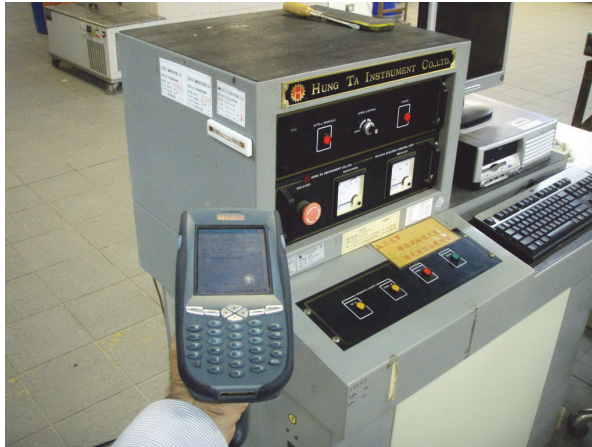
Fig. 6. Displayed maintenance staff member used RFID-enabled PDA to scan RFID tags (2).
