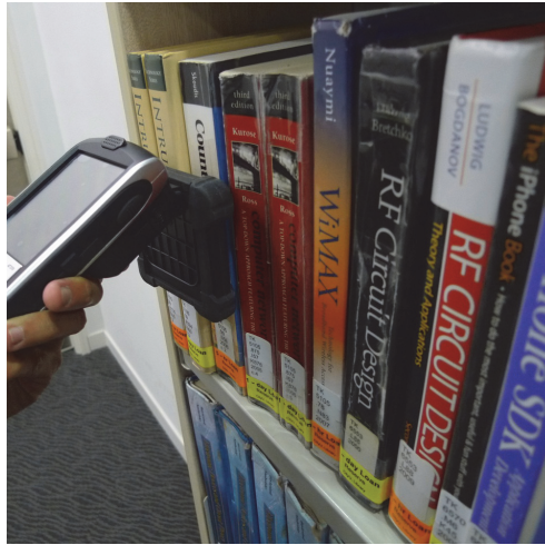
Photo 3. When books are vertically placed on the shelves, tags on the spines share the same orientation as the reader antennas in the handheld scanners while tags on the covers exhibit a perpendicular orientation.
